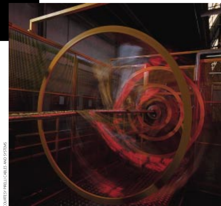
American Superconductor’s HTS tape is fabricated into a stranded conductor assembly by Pirelli Cables and Systems, using modified conventional-cable equipment. The machine on the right then wraps the conductor assembly with thermal insulation made of metalized polyester film.
