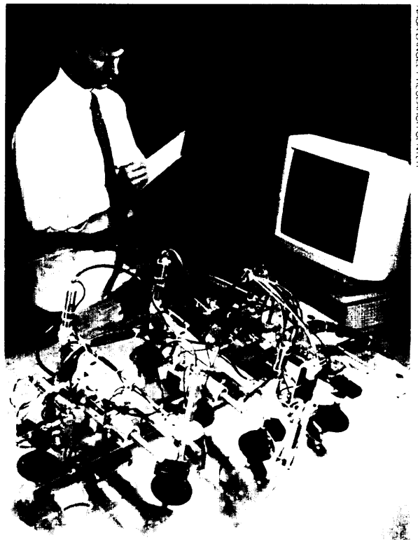
A robotic rivet inspection tool under evaluation for use in aircraft maintenance
