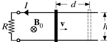
An expanding magnetic field area having a static magnetic field directed into the page produces a CCW current.
