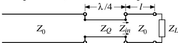
First find the reflection coefficient in order to determine the value of  $\psi$ . Then find the length  $l$  of the line that will convert the load to a pure resistance, i.e. produces the first voltage maximum. Find this resistance ( $Z_{in}$ ) using the line impedance formula. Then determine the impedance  $Z_Q$  of the 1/4-wavelength segment that will match the load to the line.
