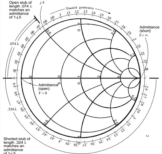
In this example, all values were in units of admittance. If we were interested in finding a stub length for a series stub problem, the units would be in impedance. The problem would be worked in exactly the same way. Of course in impedance, an open shunt (zero length) would have the value  $Z=\infty$ , representing a point at the right end of the  $x$ -axis.
