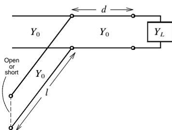
**Series-stub:** Select  $d$  so that the admittance  $Z$  looking toward the load from a distance  $d$  is of the form  $Z_0 + jX$ . Then the stub susceptance is chosen as  $-jX$ , resulting in a matched condition.
