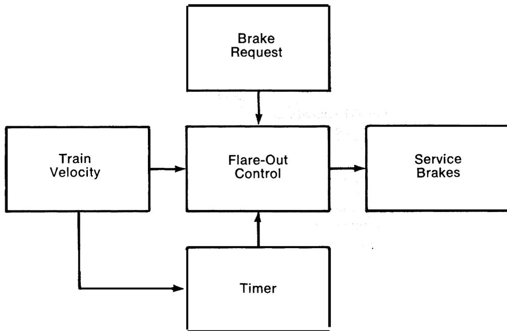
FIGURE A-3.-Conceptual Diagram of Service Brake Flare-Out Control
